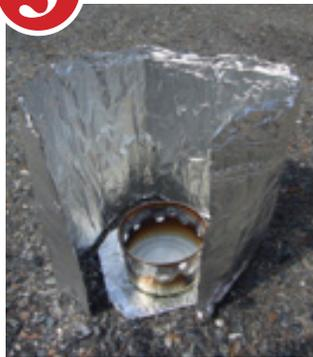
After determining the wind direction, shape the windscreen around the aluminum cup. Position the opening of the windscreen on the leeward (away from the wind) side. If there's a significant wind, you'll need to set up your stove behind a tree, rock or rise. Now place the small foil square on a flat piece on ground, inside the windscreen. Set the stove on it.
